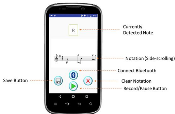
Figure 2: The user interface with some notation displayed. The currently detected note is “R”, indicating a rest.
